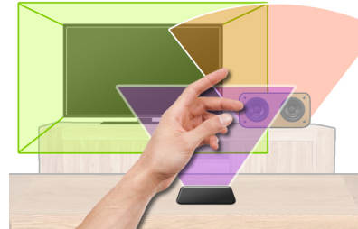
Figure 1. Users need to be able to address gesture systems, otherwise their actions may produce unwanted (or no) effects. Here, many devices are sensing input from the same space; without directing input towards one in particular, gestures may have unintended effects on other devices.
